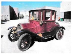
Norm built the body from blown up drawings of the Doctor's coupe as shown in the Overland brochures and parts lists. All the mechanicals are standard model 59. The wheels are 23" instead of the standard 25" for the model 59, but are otherwise identical.
